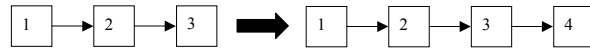
Add the new node at the end of the line. Remember to move the EOL to panel 4 OUT connection. Remember the overall cable length should not exceed 1.5km
