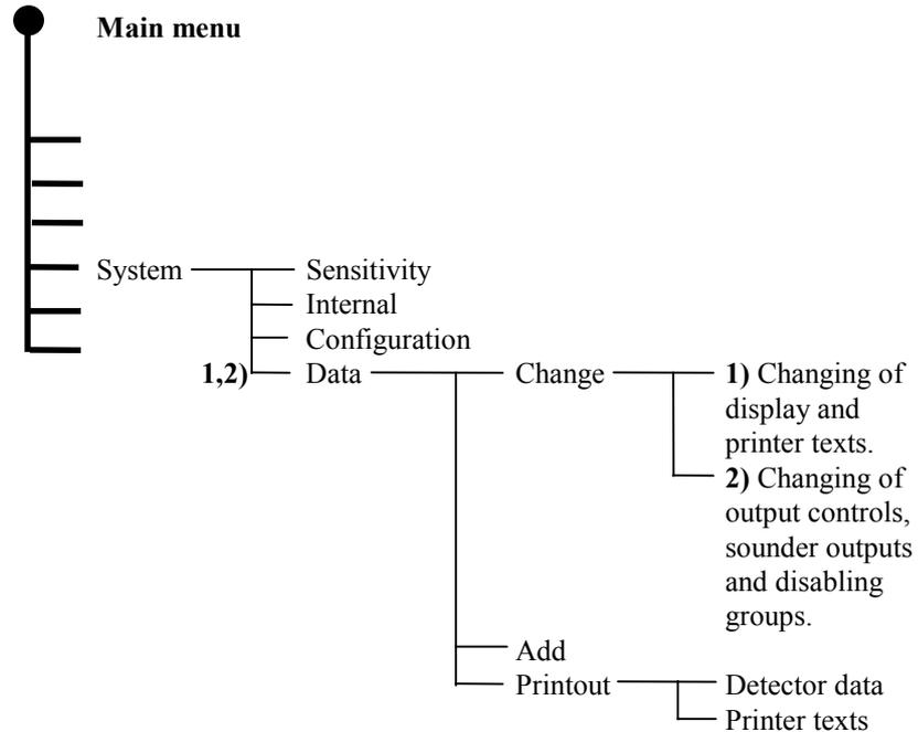
All changes and additions to custom designed text, controls, alarm outputs, groupings and printer texts can be implemented in this function. A print-out of all custom text data/site data can also be made by using this function. The function is password protected.
