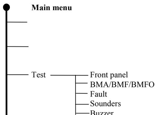
When entering the "TEST"-function in the main menu, the following text will appear in the display:
