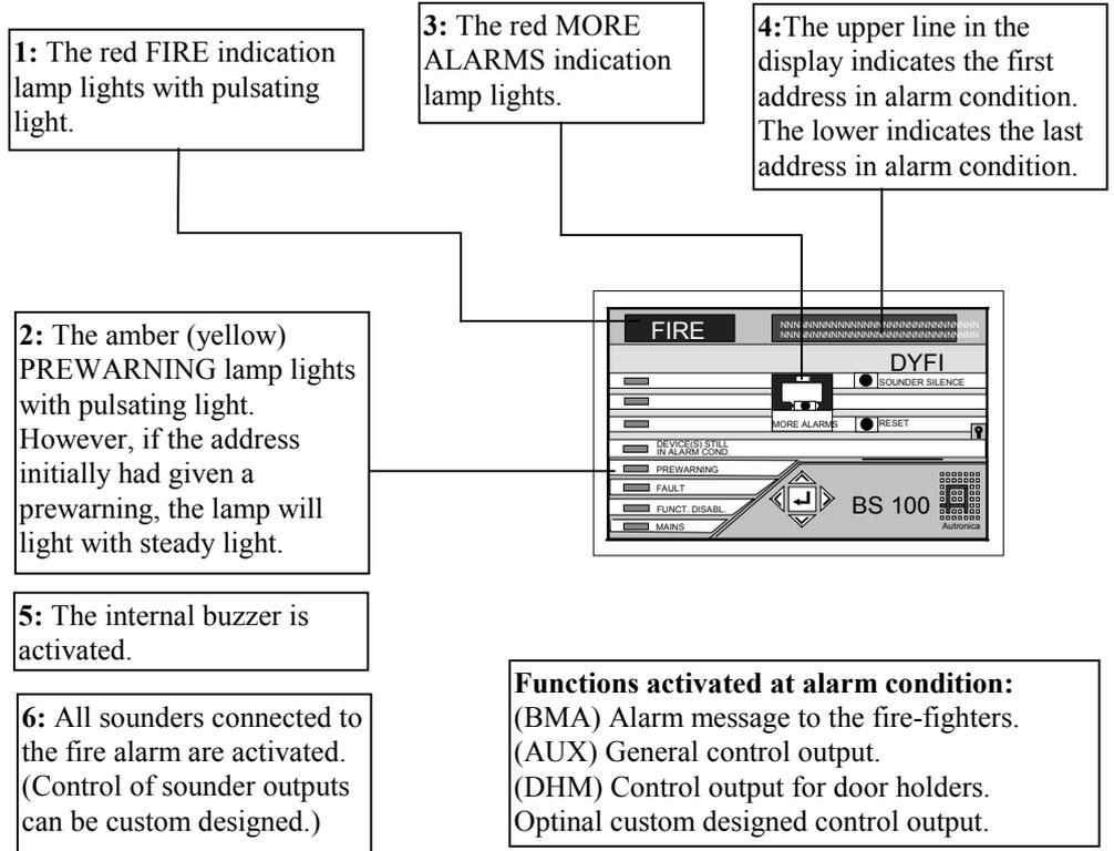
Example of text in the display if more then two detector addresses (here we show 3) are in alarm condition:
