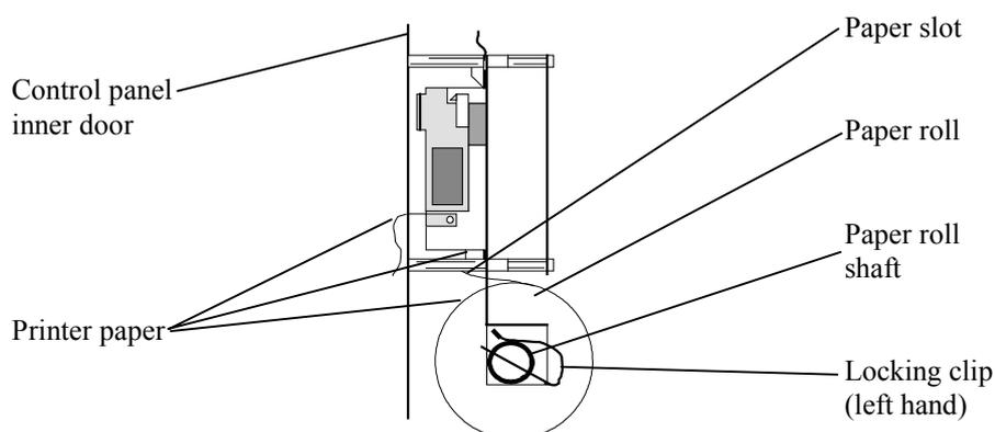
Fig. A: Side view of the optional printer located at the rear side of the inner door.
