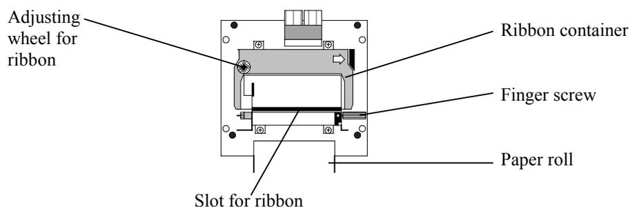
Fig. B: Location of the finger screw on the optional printer (front view).
