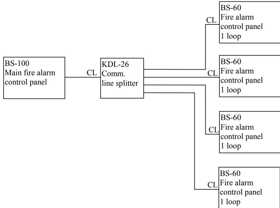
When a condition (fire, fault, prewarning) is registered on a control panel (BS-100/BS-60), the indication lamps on the panel front will light, the outputs will be activated etc. in the normal way.
