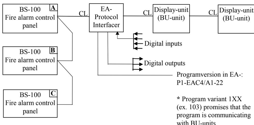
There is no communication between the individual BS-100 control panel. Each individual BS-100 control panel gives warning about its own condition and relays this to the common BU-units.
